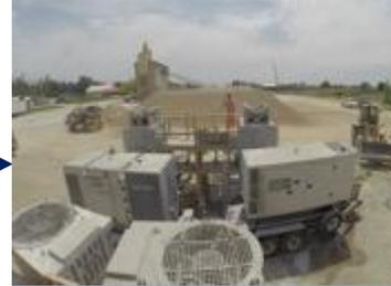
On-site plant for the manufacture of the UHPC
